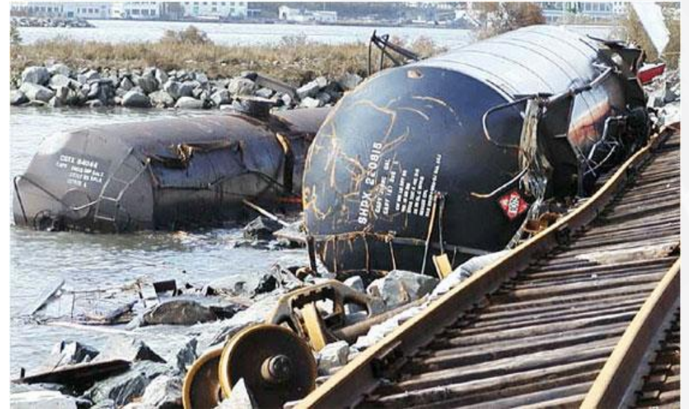
The storm surge washed out train tracks and caused these railcars to slide into Halifax Harbour, Hurricane Juan 2003 (Environment and Climate Change Canada)
